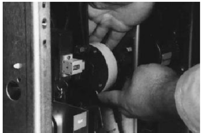
Figure 6-9 Attaching Tape Around Side of the Cam
