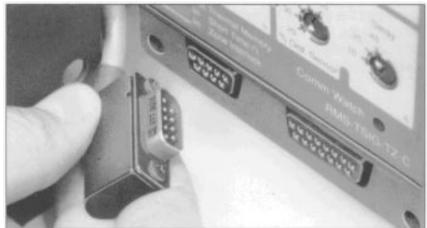
6.) Insert the BDU and/or zone interlock cables at the front of the trip unit.
