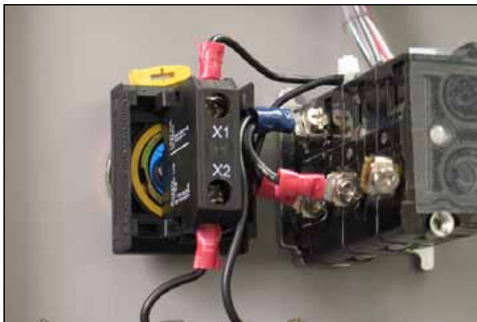
Figure 21. Indicator Light Contact Block Assembly "Locked" on the Indicator Light Housing.
