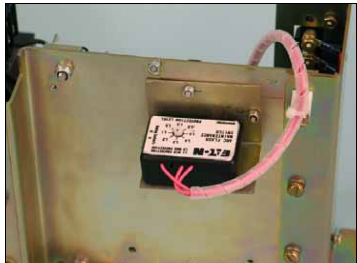
Figure 6. RSM Assembly Installed on the Trip Unit Mounting Frame.
